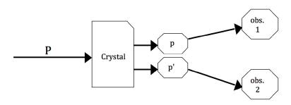
Figure 1: Set-up for observer entanglement experiment. Through the process of Spontaneous Parametric Down-Conversion, a single photon (P) is sent into a crystal and converted into a pair of entangled daughter photons (p and p'), which are then sent to separate observers (obs. 1 and obs. 2).
